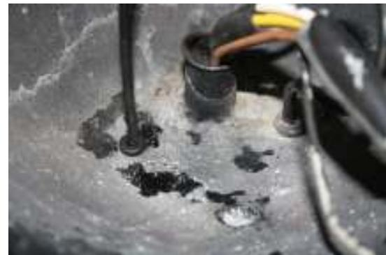
**6) \*\*Optional step\*\* (Even though the relay harness is grounded through the existing ground of the old headlight harness, a good ground is essential to proper headlight function.) You can ensure a good ground by attaching the relay harness (terminal marked optional ground) to the headlight bucket using the supplied self tapping screw.**
